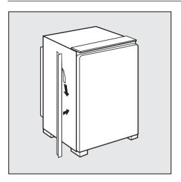
■ Stick the sealing strip to the side of the appliance on which the door is opened.
